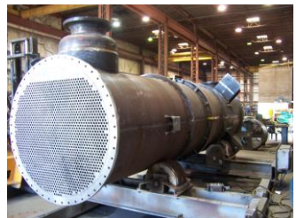
Large Heat Exchangers
