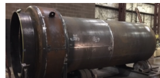
Shell for a 2,550 1" OD tube heat exchanger.
