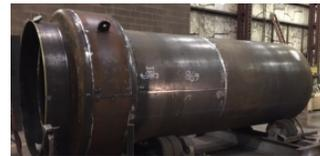
Shell for a 2,550 1" OD tube heat exchanger.
